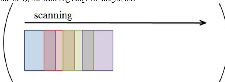
Figure 1. Illustration of the process of measuring the plate surface profile as a series of successive measurements with an overlap of about 30%.
